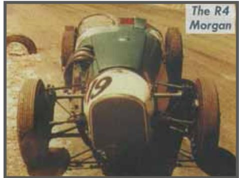
The R4 Morgan emerged after just 6 months as an open-wheeled racing car. The Plus 4's rather flexible chassis had been replaced with a highly rigid tubular space frame incorporating the original front end, which was widened by 2 inches and had Austin A40 stub axles grafted on. A Peugeot 203 rack and pinion steering box and locally made, finned, alloy brake drums based on those of a Fiat 1300 replaced the originals.
