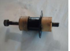
Mount casing with end pieces and bolt in place for making rear gearbox mount
