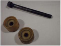
End pieces and bolt used as mould for rear gearbox mount
