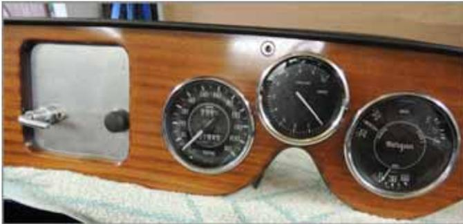
The dashboard is out of the car on the work bench and I have fitted a Smiths rev counter in the centre
