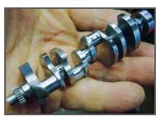
The finished 1/6 scale 5-bearing crankshaft fits into Jim's hand. It utilizes real Babbitt bearings.
