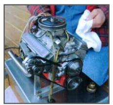
These models are built by craftsmen in the same way that the big ones are made by machining billet stock and castings.
